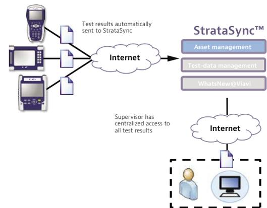
Figure 5. Test-data management using StrataSync
