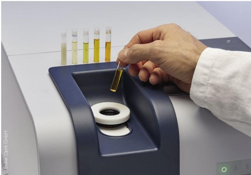
infrared region of the electromagnetic spectrum and convert this energy into molecular vibrations. Since each molecule is constructed differently and has characteristic vibrations, different ranges of IR radiation can also be
