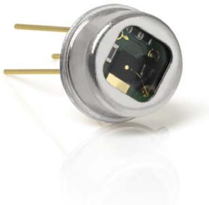
The coating works in a similar fashion to an anti-reflection coating. Data shows that over the spectral range of 2–25 microns, 93% of the incident infrared is absorbed. This approach significantly improves the performance of lithium tantalate devices at high frequencies. From our research and production facility in Arizona we supply customers all over the world with these industrial grade thermal detectors. ■
