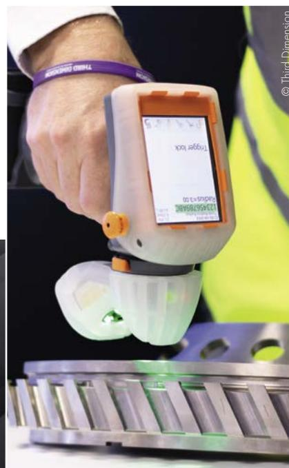
The portable gap measuring system GapGun with laser triangulation considerably reduces the working time and the costs of the manufacturing processes.
