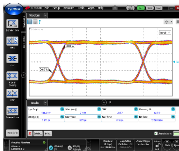
Input signal Eye amplitude = 0.45 V pp
