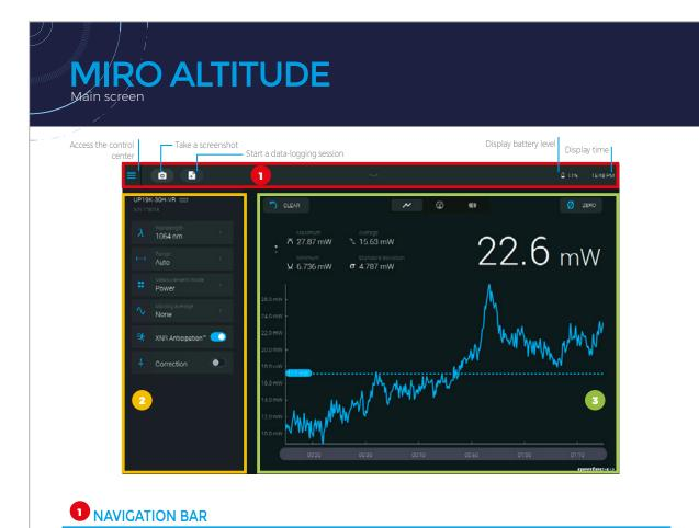
The upper part of the screen includes a direct access to the control center, data acquisition buttons and various indicators (battery level and time).
