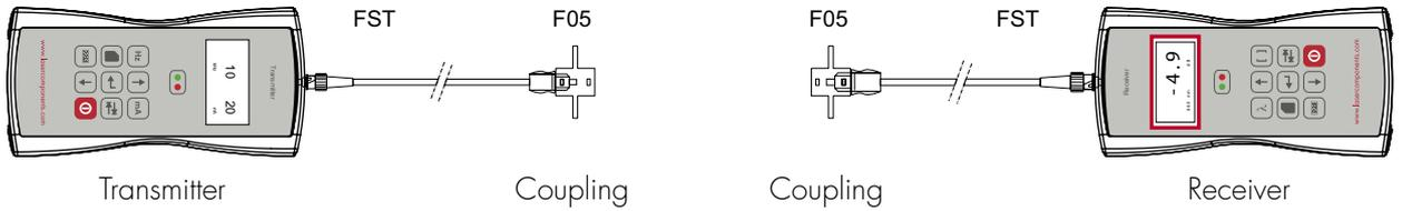
**Test Sequence Step 4:** Attenuation measurement of the test sample
