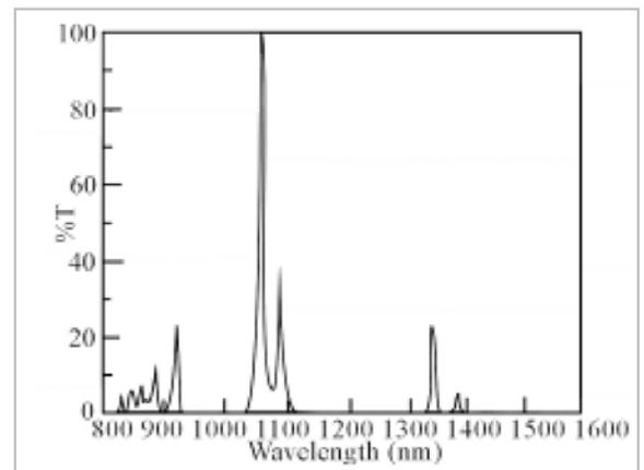
Normalized fluorescence spectra from 800 nm to 1600 nm of Nd 1.1 at. % doped Nd:YVO<sub>4</sub> for  $\pi$  polarization (a) and for  $\sigma$  polarization (b).
