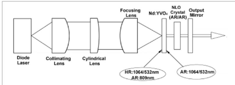
Basic experimental scheme of diode laser pumped Nd:YVO<sub>4</sub> green laser
